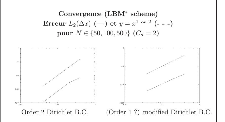
Thus, the modified Dirichlet B.C. seems to be of order 1. This B.C. is adapted when the mesh is rough (*cf.* porous medium) since the max. principle is verified (ROBUST code). But, when the mesh is fine, the order 2 is better. <u>Test-case 3:</u> Influence of the first iterate  $\rho_i^{n=1}$  on the properties of the Du Fort-Frankel scheme
