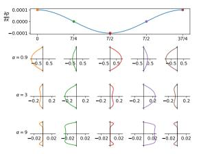
Temporal evolution of the pressure gradient (top) and the corresponding velocity profile  $u_x(y,t)/U_0$  for different values of the Womersley number  $\alpha$ .
