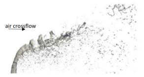
Numerical simulation of a kerosene flow destabilized by a crossflow of air
