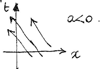
$$\begin{cases} \frac{\partial u}{\partial t} + a \frac{\partial u}{\partial x} = 0 & t > 0, x > 0 \\ u(x, 0) = u_0(x) & t = 0, x > 0 \\ u(0, t) = v_0(t) & t > 0, x = 0 \rightarrow \text{u-limite} \end{cases}$$
