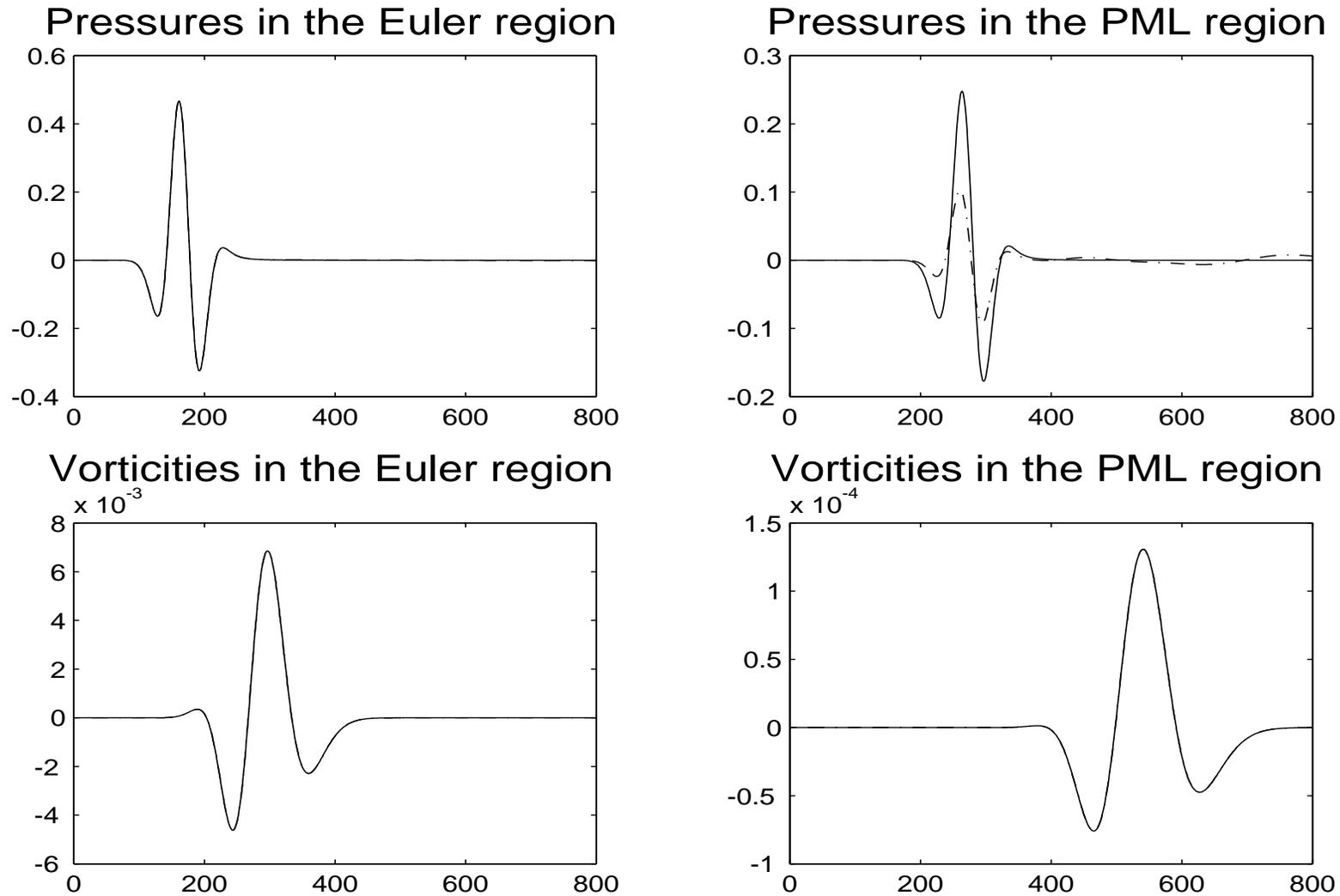
Figure 2: Reference and “PML” solutions in the Euler and PML regions vs. time steps ( $\bar{u} = 200$ ,  $\bar{v} = 100$ )
