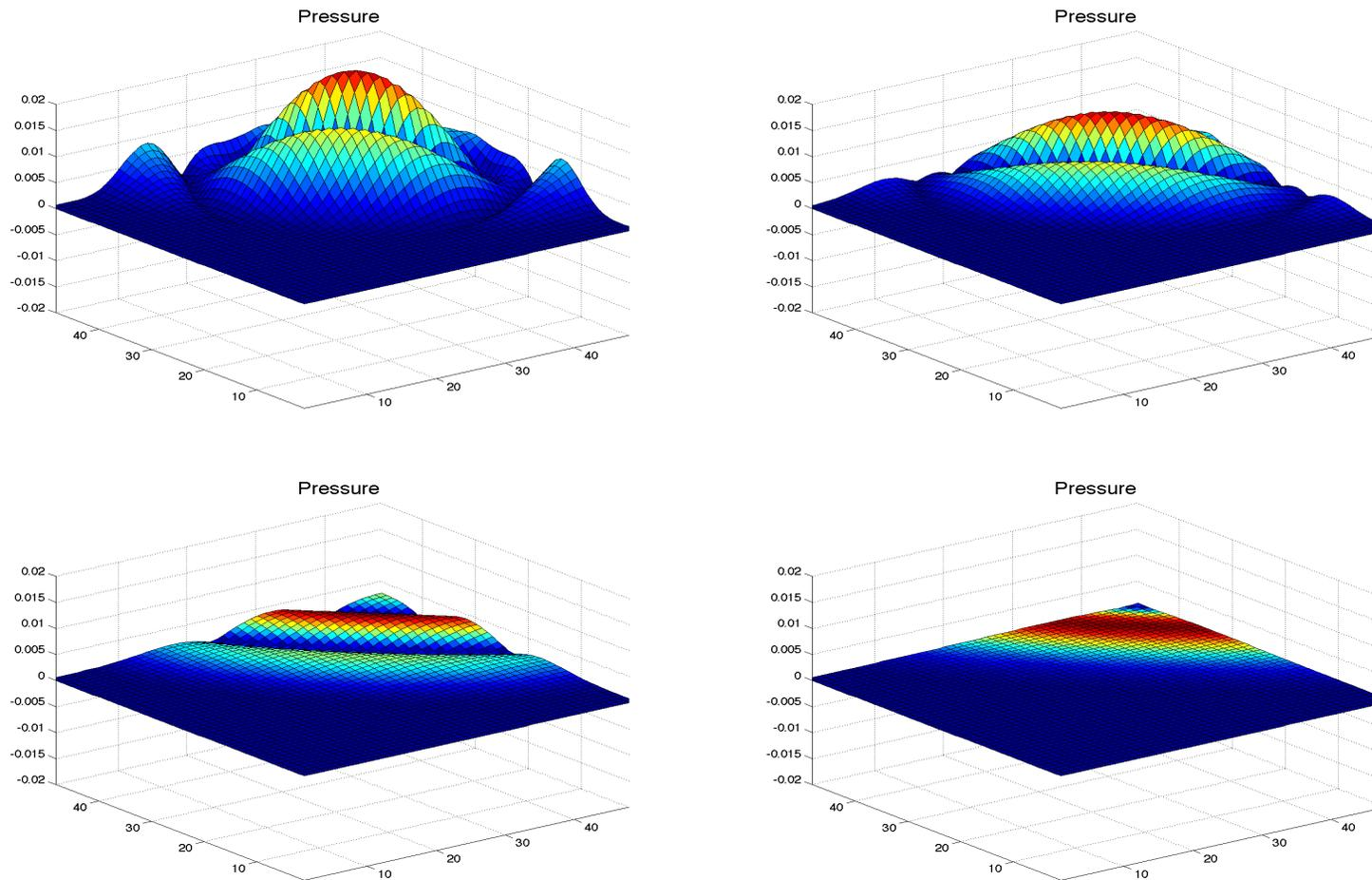
Figure 1: Pressure – oblique velocity  $M = 0.9$  at successive times
