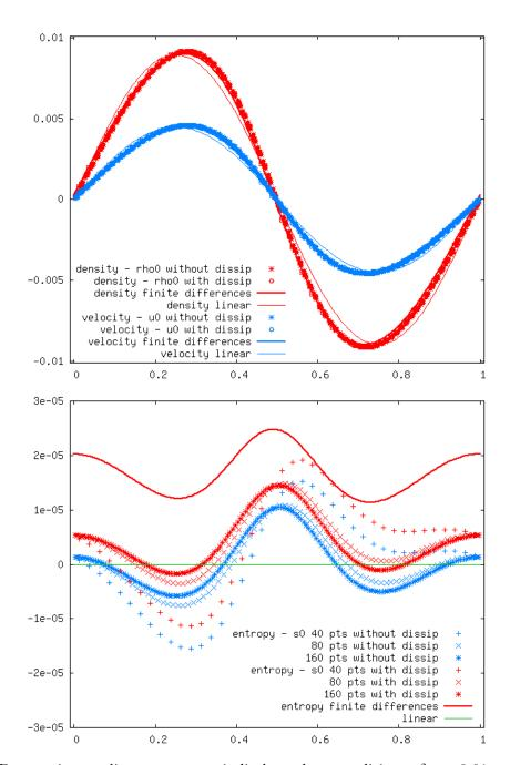
Figure 2. Progressive nonlinear wave, periodic boundary conditions,  $\delta \rho = 0.01 \, \rho_0$ . Density and velocity (top). Entropy (bottom).
