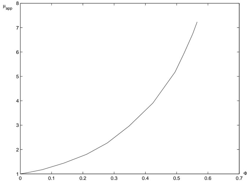
Figure 4 : Apparent viscosity with respect to solid fraction for uniform distributions.
