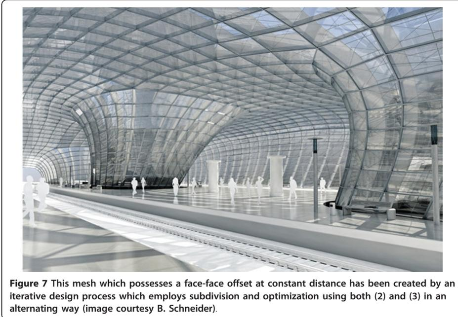
**Figure 7** This mesh which possesses a face-face offset at constant distance has been created by an iterative design process which employs subdivision and optimization using both (2) and (3) in an alternating way (image courtesy B. Schneider).
