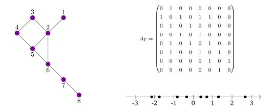
Figure 1: A (simple, unoriented) graph, its adjacency matrix and its spectrum.
